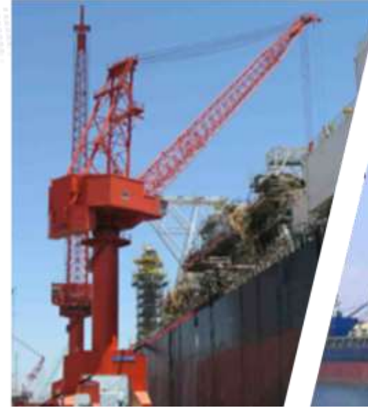
Gemi Tamir Portal Vinci Ship repair gantry crane
